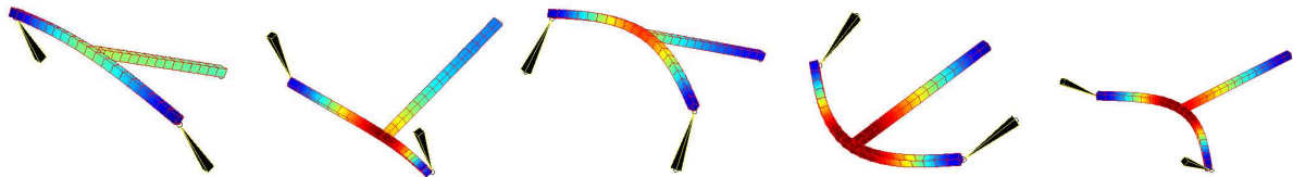
Figure 1: Motion and deformation of the spatial slider–crank mechanism.
