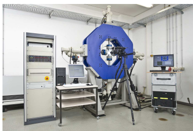
Hydraulic biaxial machine
